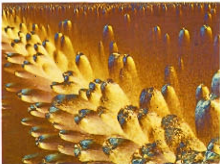
Fig. 99: Plastic substance (fault) Microtome section ORTHOLUX POL BK Objective NPI 6.3/0.20 P
