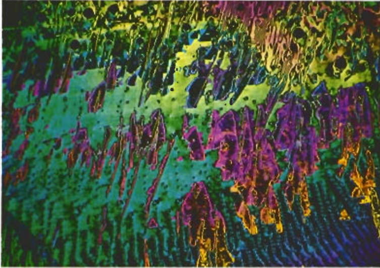
Liquid crystal (MBBA) ORTHOPLAN POL., objective NPI 6.3/0.20 P 9x12cm large-format camera
